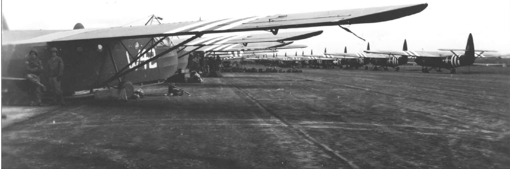
HACKENSACK - June 7 th - Gliders marshaled for take-off at Upottery Field, England 6 June, CG-4A WACO gliders are at 45 degree angle on the left of the runway, Horsa gliders on on the right, nose to tail. The loading at the time of the photo was in progress. These are the gliders towed from Upottery to Normandy on 7 June 1944 by the 439th Troop Carrier Group. On board were members and equipment of the 2nd Battalion of the 325th Glider Infantry Regiment (GIR) and most of the attached 2nd Battalion of the 401st Glider Infantry, 82nd AB Division.
